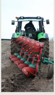
true is that the top-link is in line with the plough and tractor.
